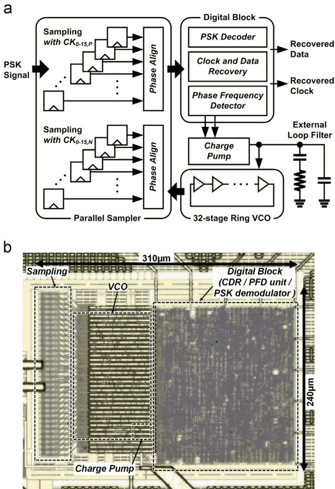
Fig. 4. (a) Block diagram of prototype demodulator. (b) Die photograph of prototype chip.
