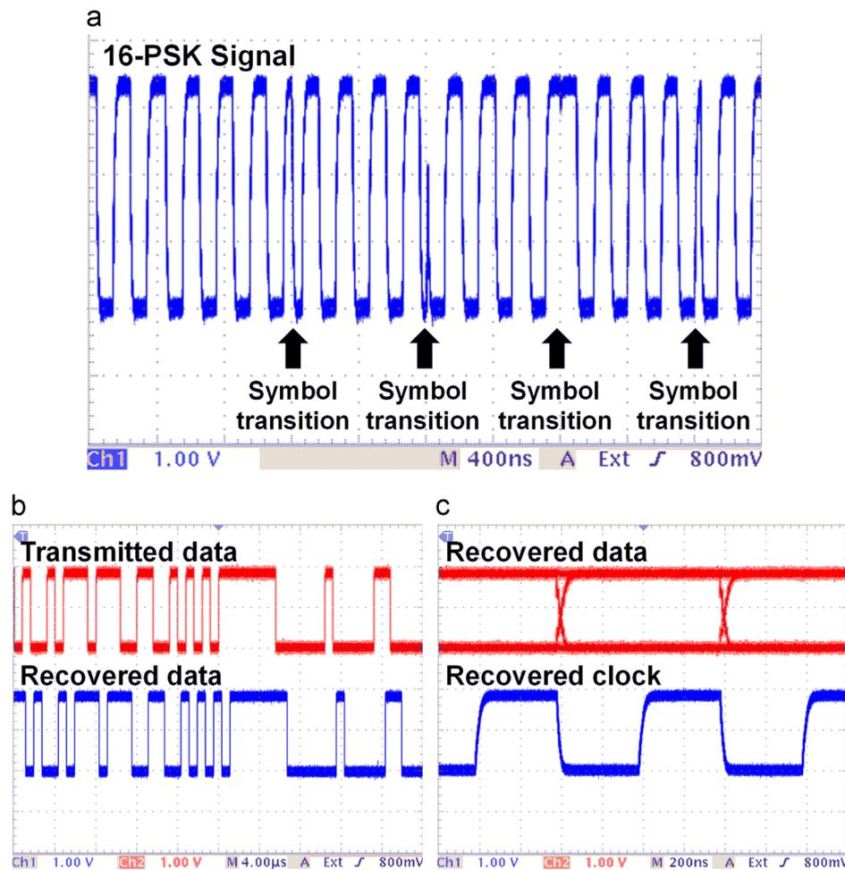
Fig. 8. (a) 16-PSK signal used as the input of the prototype chip. (b) A pair of 4 transmitted and recovered data streams for 16-PSK in inductive link. (c) Recovered data eye-diagram and recovered clock. (I/O supply: 3.3 V).
